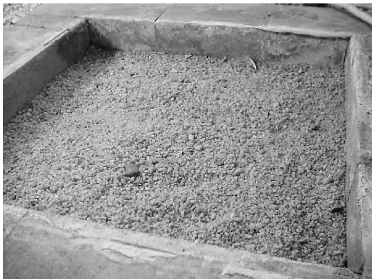
Fig. 16. Cleaned debris by in situ thermal desorption.
